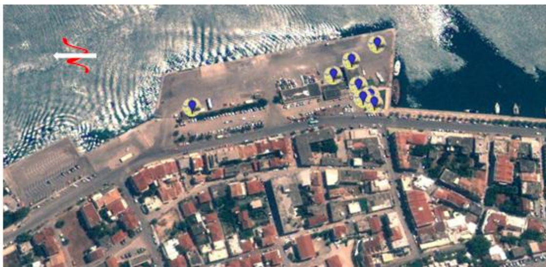
Figure 2.21. General outline of liquefaction traces recorded after the second earthquake along Argostoli port.
