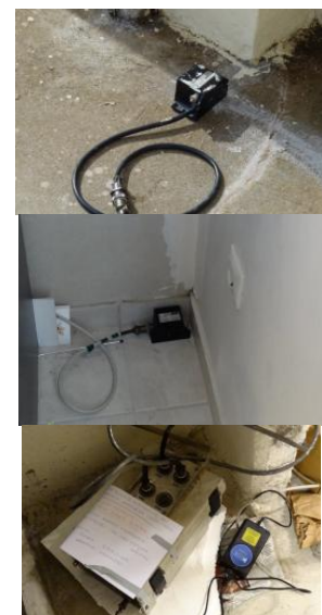
Figure 3.1. The administration building of the Lixouri Hospital (left) and photos from its instrumentation with the special accelerometer array (right).
