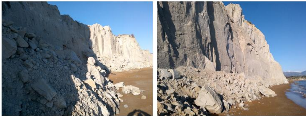
Figure 2.5. Shoreline of Xi area (from 38.159537^{\circ} N, 20.410148^{\circ} E to 38.160405^{\circ} N, 20.413083^{\circ} E) south of Paliki peninsula where an extended slide (almost 250m long) of a sandy marl escarpment was observed.
