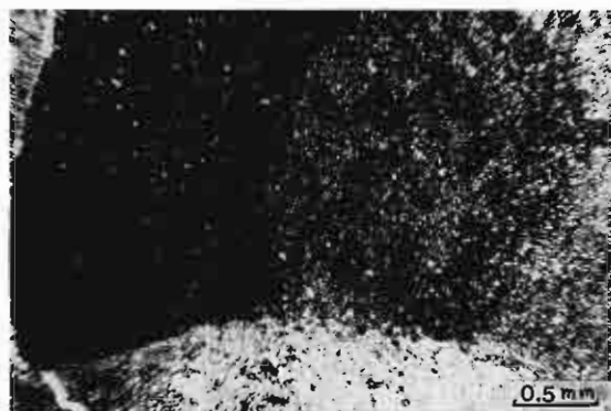
Figure 18. Phytoclast differentiated to an external part consisted of concentric coatings and an internal part, consisted of amorphous opaque material.
